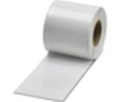
Marking foil for zack marker strip, Roll, white, unlabeled, can be labeled with: THERMOMARK ROLL 2.0, THERMOMARK ROLL, THERMOMARK ROLL X1, THERMOMARK ROLLMASTER 300/600, THERMOMARK X1.2, mounting type: adhesive, for terminal block width: 30000 mm, lettering field size: 30000 x 3.8 mm, Number of individual labels: 1
