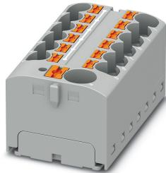
Distribution block, nom. voltage: 450 V, nominal current: 32 A, connection method: Push-in connection, Push-in connection, number of connections: 13, cross section: 0.2 mm<sup>2</sup> - 6 mm<sup>2</sup>, AWG: 24 - 10, width: 46.3 mm, height: 21.7 mm, color: gray, mounting type: for snapping onto a DIN rail adapter, Direct mounting with flange, Free-hanging
